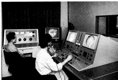
FIG. 6. Photograph of the control room of the present x-ray television unit.
